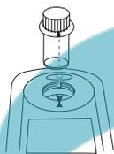
Place the prepared sample vial in the sample chamber making sure that the positioning is correct, with the index marks aligned.
