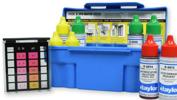
The K-1004 6-Way DPD kit monitors three variables that impact water quality so problems can be detected and treated early, with less expense.
